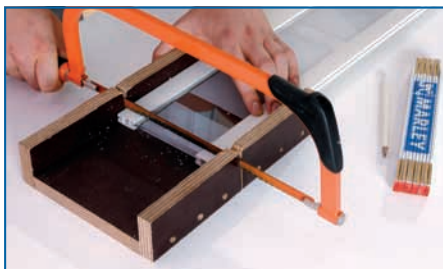
Cut the profile to the required length
